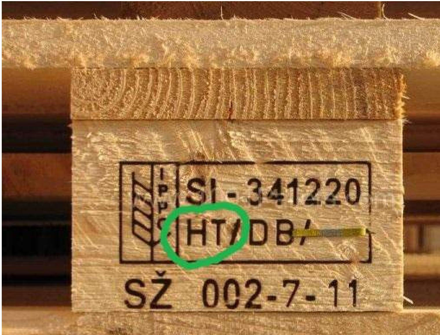
**HT= Heat treated, the better alternative for insect control for imported wood**
